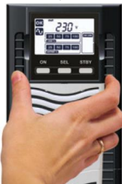
1. Remove the display panel
