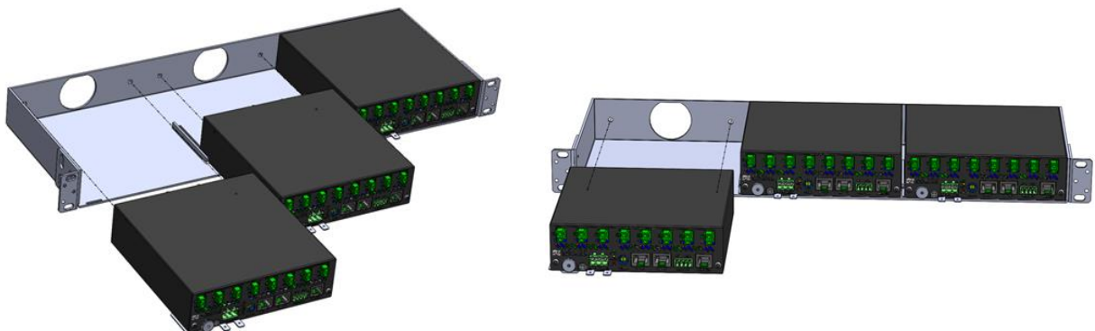
DC/DC-TPU-120-48 and DC/DC-RPU-120-48 modules installation in the 19"/21" shelf
